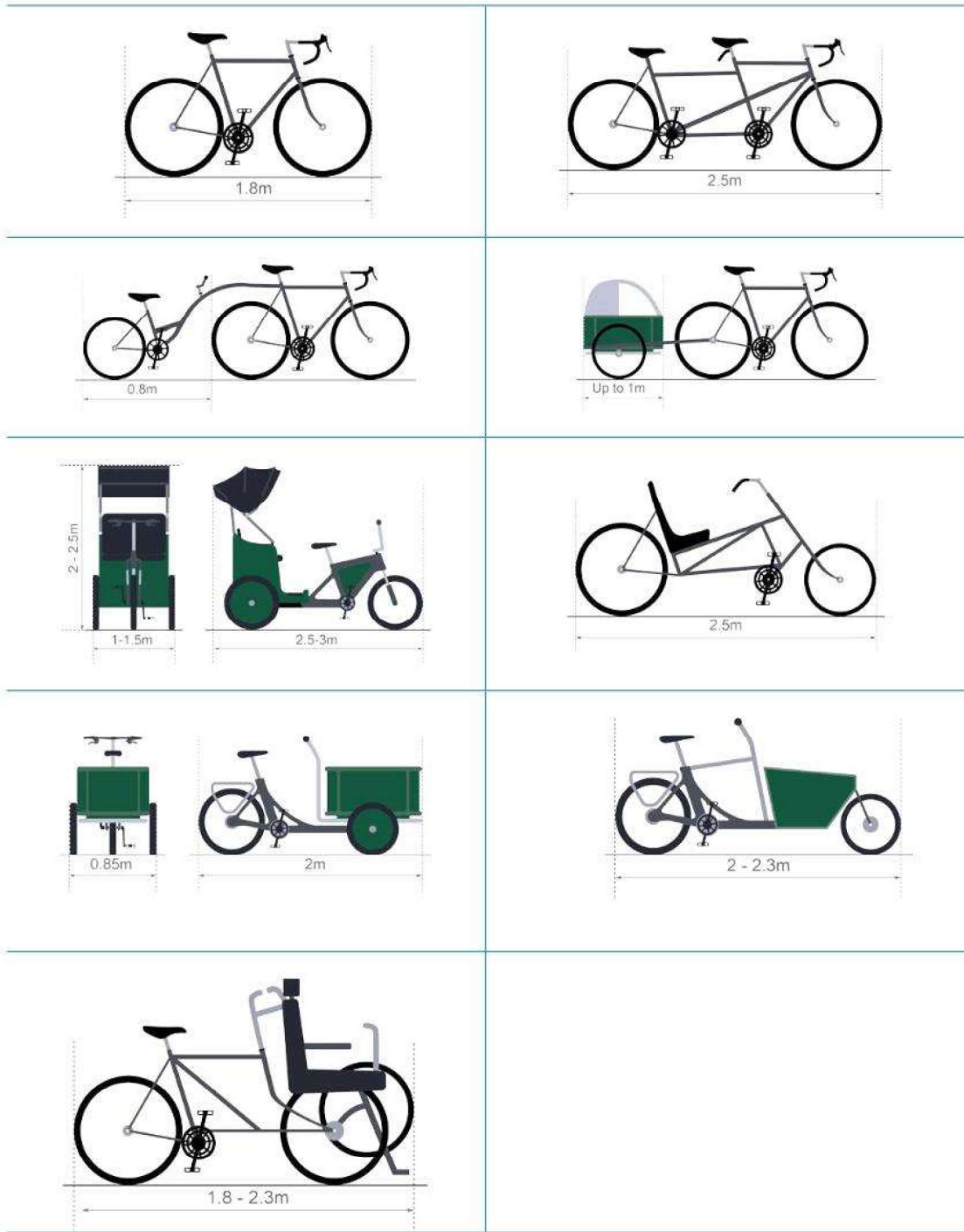
© LTN 1/20, Department for Transport Figure 6 Cycle users and widths
